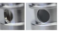
Example: before with burring, after completely free of burrs
